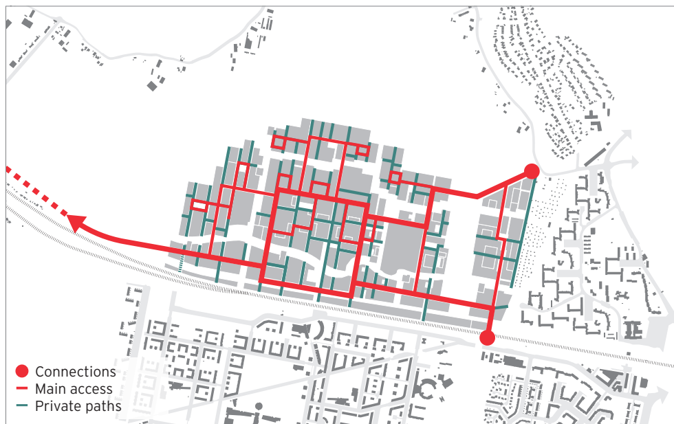
Differentiated road network in the district, with three access connections
