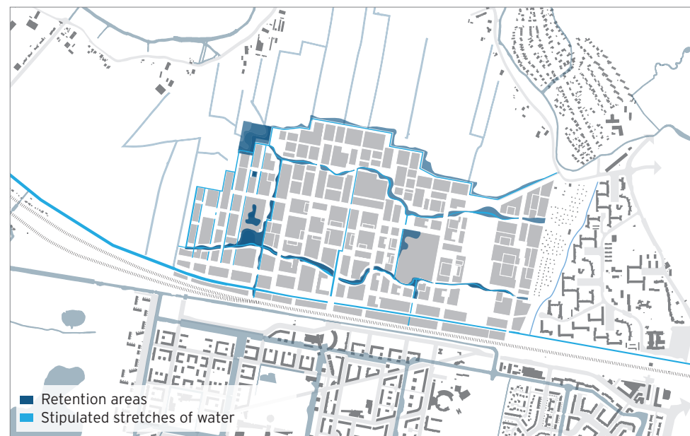
Large retention areas enable the safe retention of water from heavy rainfall events
